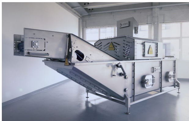
Figure 8 An industrial pulsed electric field apparatus for pre-treatment of solid materials (Elea, Germany) [89]
