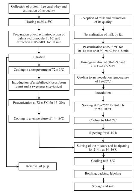
Fig. 1. Process chart for the production of Lesnoi kefir beverage.
