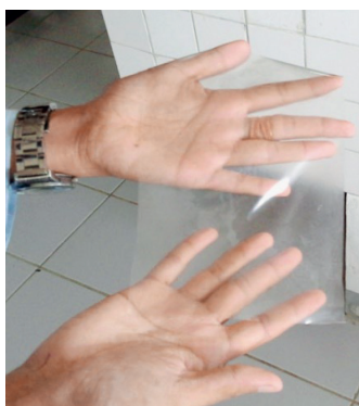
Figure 1. Biodegradable plastic from 10% banana peel starch and 5% glycerol
